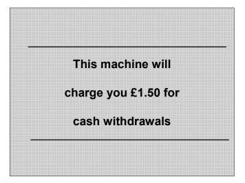
For medium-sized screens (between 171mm and 200mm wide) the minimum font size is 26, and the message must cover 60% of the screen.
